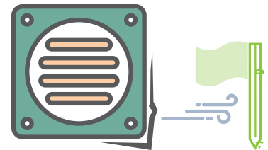
Wall Air Leak (caulking can be used to seal gaps or cracks)
